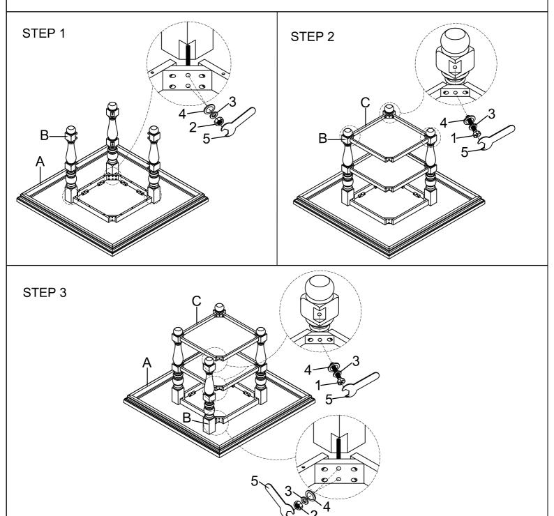
Step 1: Turn Table Top (A) on the floor with a piece of cloth or carpet underneath to prevent finish from scratching. Attach Leg (B) to Table top(A) and assemble by inserting Flat washer(4), Spring washer(3), Hex nut (2), then tighten with Wrench (5). Repeat the same steps for the other two legs. Do not fully tighten.
