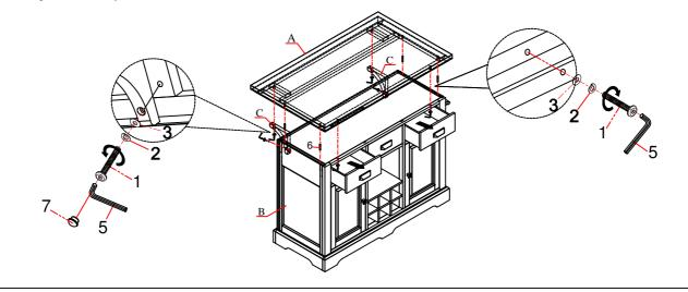
Step 2: Attach the Pull Handle (D) to the Base Cabinet (B) by using Wood Screw (4). Secure well by the screwdriver. Complete by attaching Leveler to the four corners of the Cabinet (B) bottom.
