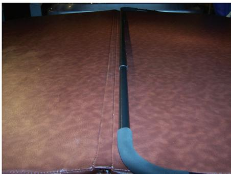
**Step 5** – Lay the cover lifter on the spa cover, adjust the coupler piece and support arms so that the coupler piece is lying parallel to the spa cover's hinge about a 1/2" away. Using the #10 self tapping screws, fasten support arms to pivot arms and the coupler piece.
