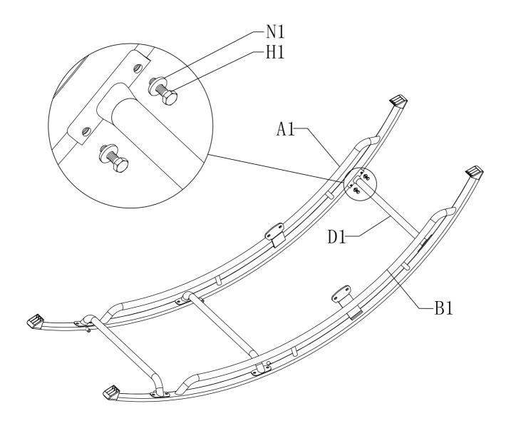
Friendly Tip: Please don't completely tighten the screws during assembly. After all the screws are assembled in place, tighten them together.
