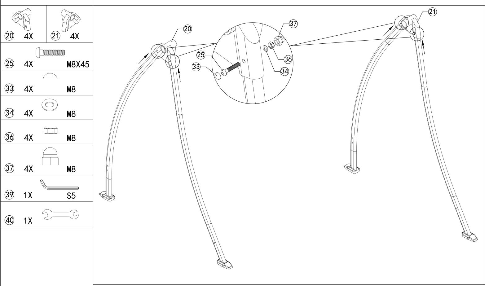
Step 2: Put the front and rear leg tubes (Part 1 is front leg tube, Part 2 is rear leg tube) into the fixator (Part 20 and Part 21) as shown, and secure with bolts and nuts as required (After all the bolts are assembled in place, tighten them together, finally cover the caps).
