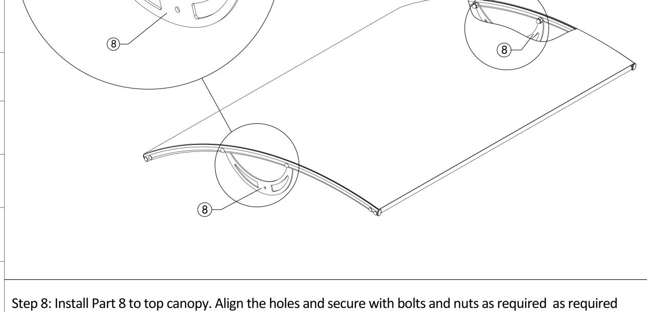
(After all the bolts are assembled in place, tighten them together, finally cover the caps).
