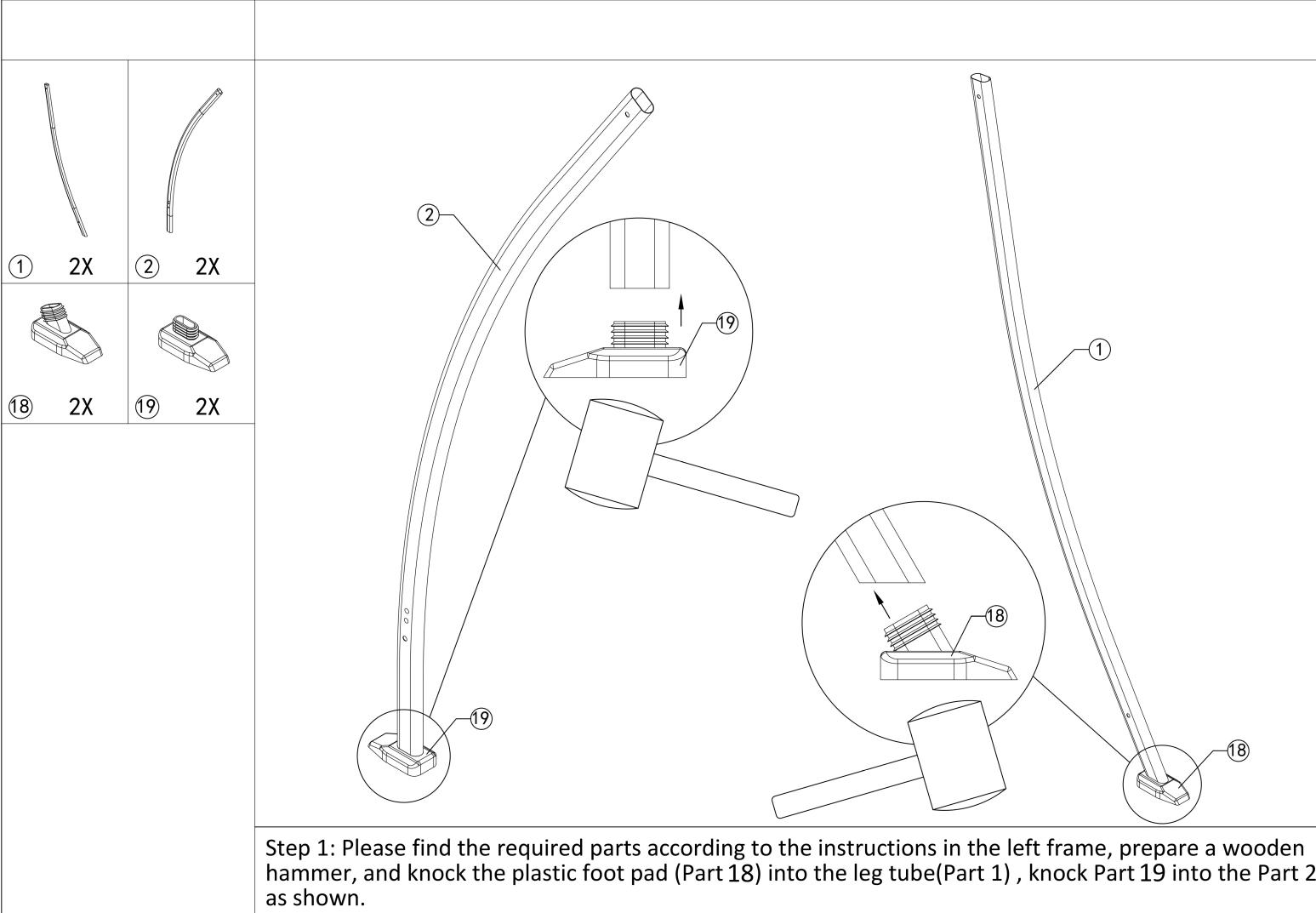
hammer, and knock the plastic foot pad (Part 18) into the leg tube(Part 1), knock Part 19 into the Part 2
