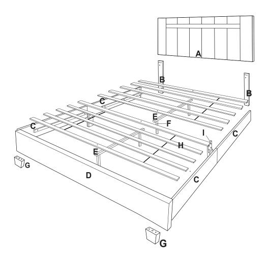
Bed Parts are shipped inside a compartment in the back of the headboard & footboard.
