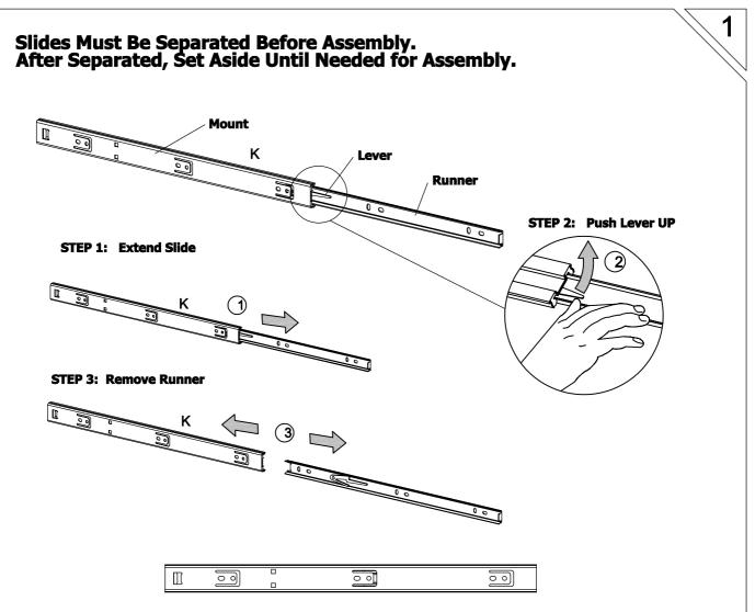
When installing the outer guide rail, please use the guide rail notch to assemble towards the inner direction of the drawer. Please fix the screws according to the marked position. If the installed position is changed, adjust it side-to-side at the marked position.
