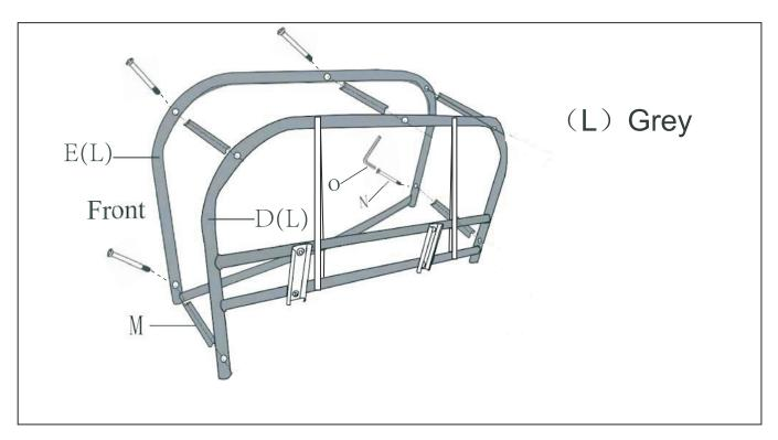
STEP 2:Align the armrest cover to armrest-assembled iron frame in sequence of left and right, back and forward. so that the cloth cover hole is aligned with the insert hole. Pull the zipper after all is OK.
