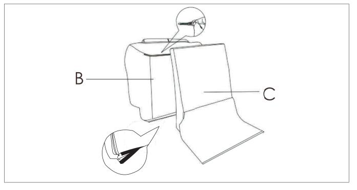
STEP 9 :Plug the back pad into the seat frame, and then connect the massager line white and white, red and red, black and power lines, and the massage line with the hand controller.
