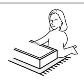
NOT TO BE INSTALLED ON HARD GROUND!PLEASE USE CARDBOARD OR CARPET AS A BUFFER LAYER DURING THE INSTALLATION!
