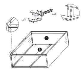
Put ⑥ in the designated position and fix it with four screws A.
