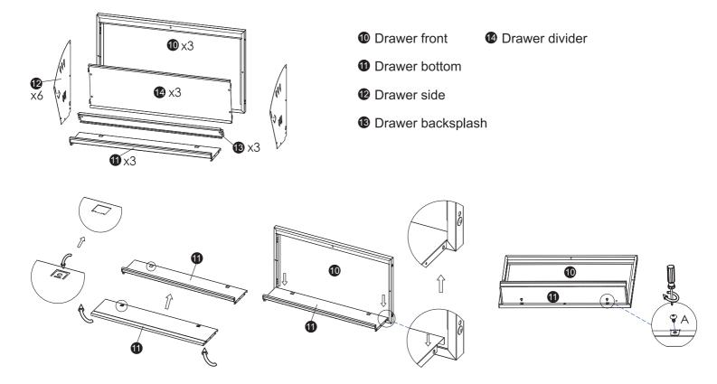
Bend the front end of (1) upwards, the back metal buckle downwards, and then clamp it to the bottom of (1).
