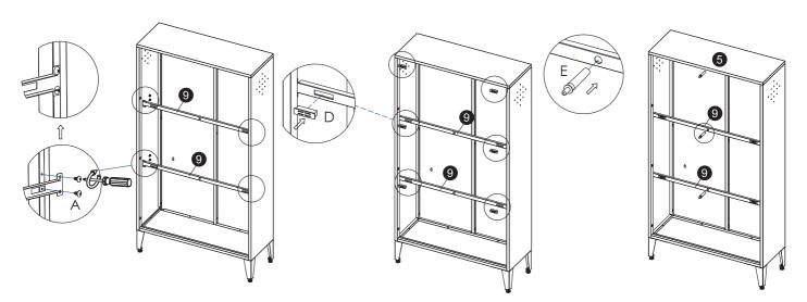
Install two @s at the positions as shown in the figure, and fix them with 8 screws A. Then insert D into both sides of the top and @.
