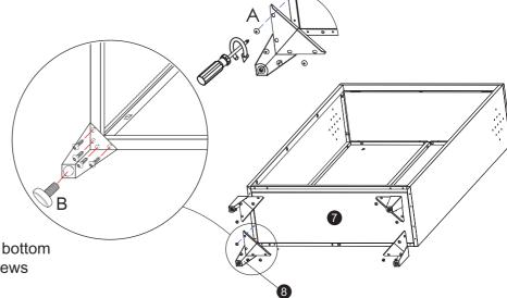
Lay the cabinet down, align @ with the bottom screw holes on @, and fix it with 16 screws A.Then rotate to install B.
