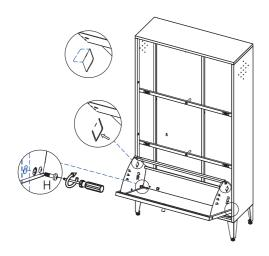
Install the assembled drawer on the shoe cabinet, and install two screws H to fix both sides. Then bend the metal buckle on ② outward to prevent the drawer from falling, as shown in the figure.
