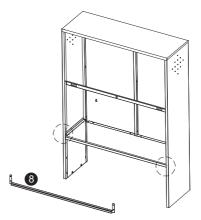
Place (8) in the bottom position (as shown), then align the screw holes, and fix it with 4 self-tapping screws (B).
