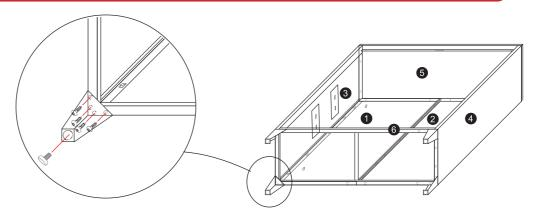
Align the holes at the bottom of ⑦ and ⑥, as shown in the figure below, install and fix them with screws (B\*4 pcs), and screw the foot pads (E\*1 pcs) into the holes at the bottom of ⑦, and use the same for the other three At the same time, fix the two holes in the middle of the bottom of ⑥ with screws (B\*2 pcs), and then erect the cabinet.
