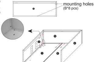
Put ⑤ on top of the U-shaped frame, align the bottom hole with the hole on top of the U-shaped frame, and fix it with screws. (need to use B\*8 pcs)
