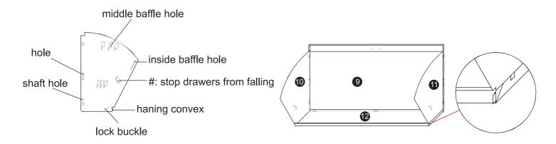
Pry the 6 metal buckles on both sides of 9 inward by about 45°, and insert the mounting ears at the bottom of (1) into the hanging holes of (12), as shown in the figure (note that (11) is on the inside of (12)), align the metal buckles of 9 with the holes of 10, and then upward Press the metal button, and then press the lock into the corresponding lock hole, so that ① and ② are locked, and ① is installed in the same way.
