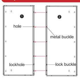
Lift the five metal buckles on ② outward by about 45° and insert them into the corresponding holes of 1, press the metal buckles down, and press the lock buckle on 2 90° to the left to lock 1 and 2.
