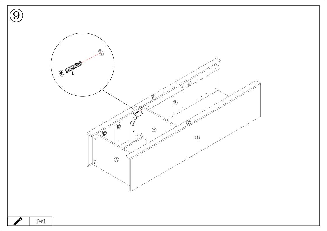
Make sure the arrow on the screw align to the hole on the side. 1 3 (5) put B on board **348** B**\***5
