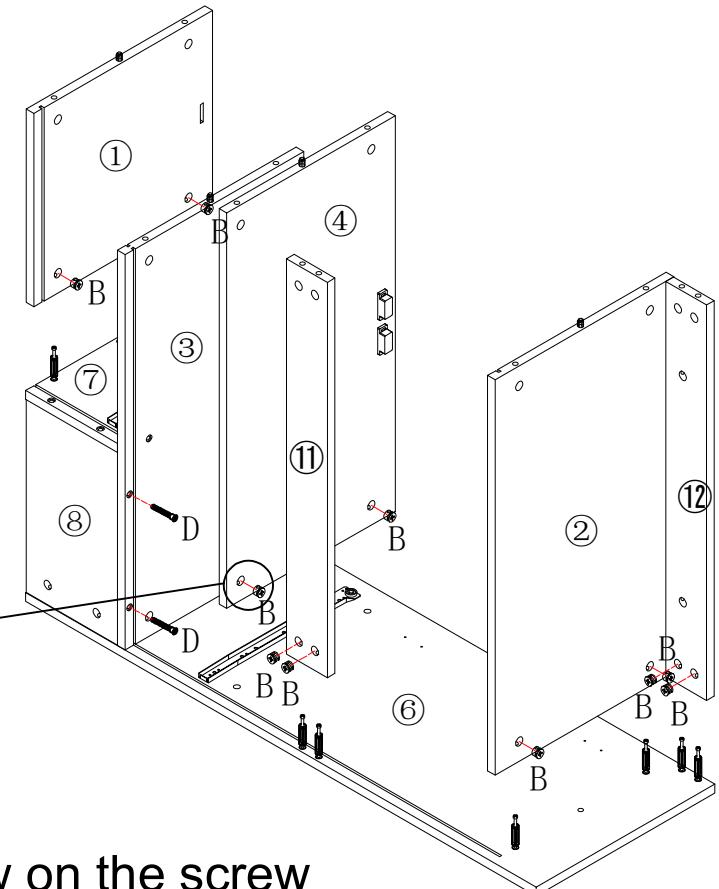
Make sure the arrow on the screw align to the hole on the side.
