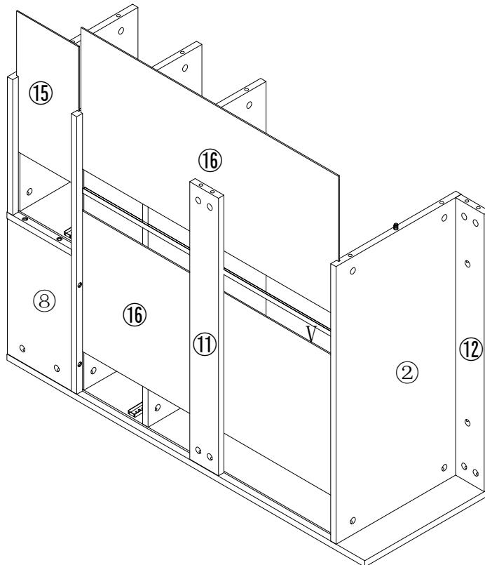
Make sure the arrow on the screw align to the hole on the side.
