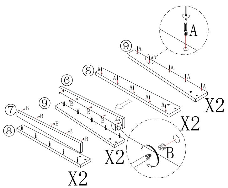
Make sure the arrow on the screw align to the hole on the side.
