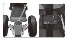
Remove the two screws on the seat plate, open the seat plate, remove the battery socket plastic protective cap, the red plug at the battery red socket plug that the total power is connected.
