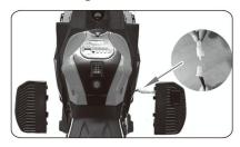
Take the pedal, first connect the pedal line, and then the pedal is installed to the corresponding position of the car body, clamp can be
