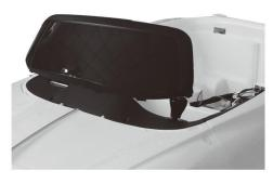
3. Install the front windshield: The windshield is aligned with the card port on the body and is forced in.
