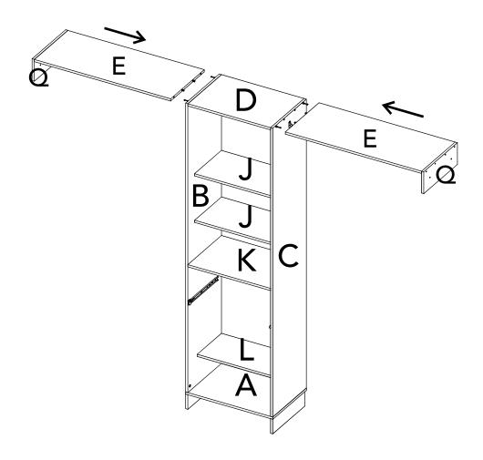
**1** You must drill the bottoms guided by the holes in the structures wiht a 3/16" drill bit.
