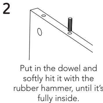
Put in the dowel and softly hit it with the rubber hammer, until it's fully inside.
