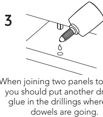
When joining two panels together, you should put another drop of glue in the drillings where the dowels are going.
