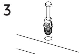
This is a spreading bolt. You should put it with the black plastic part facing down.
