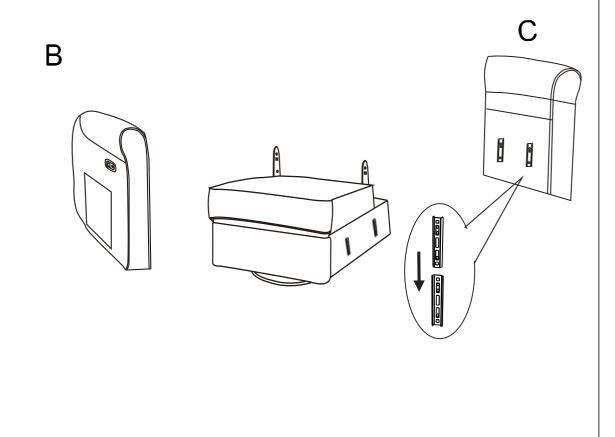
Ensure the backrest (A) slides down fully over the brackets on the seat(D).
