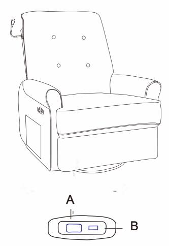
Press the A button to reline the chair B button is use to connect USB
