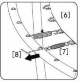
Pull the Spring Tool(#8) until the spring hook insert the hole on the Top Rail and disengage the Spring Tool(#8) leaving the Spring (#7) In place.Repeat process for all springs
