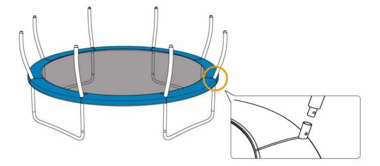
Insert the Up Safety Pole(#12) into the top of the Bottom Safety Pole(#11), and then rotate the Up Safety Pole(#12) to make the hole position coincide with the marble position of the Bottom Safety Pole (#11) untill the metal marbles pop out and fixed. Repeat step 7 to install 6 of the safety pole
