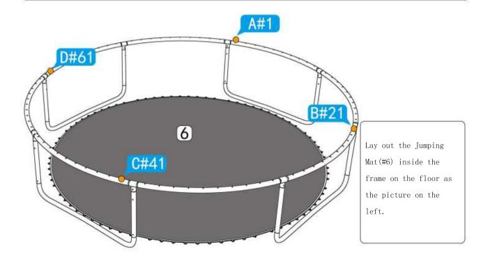
When assembling the jumping mat, please make sure to attach the jumping mat with 4 symmetrical point fixed into the frame first. Then install springs symmetrically every 3 holes along the 4 fixed point.
