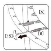
Pull the Spring Tool(#15) until the spring hook insert the hole on the Top Rail and disengage the Spring Tool(#15)leaving the Spring(#8) In place. Repeat process for all springs.
