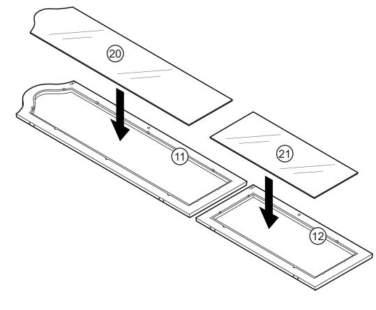
Secure the cabinet door glass panels in place.
