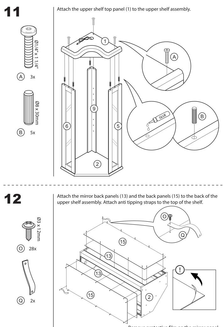
Remove protective film on the mirror panel.
