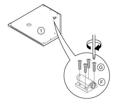
Attach the cabinet light socket to the underside of the upper shelf top panel (1).
