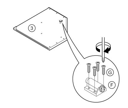
Assemble the lower shelf top panel (3) on top of the lower shelf assembly.
