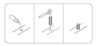
APPLY GLUE INTO PRE-DRILLED HOLE, AND GENTLY TAP WOOD DOWEL INTO THE HOLE WITH RUBBER MALLET.
