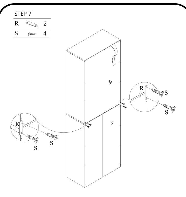
The two cabinets can be connected with Connecting Pieces.
