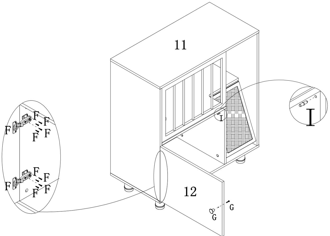
**EN** It may be necessary to adjust the hinges so that the doors align. Use the instructions below as a guide.
