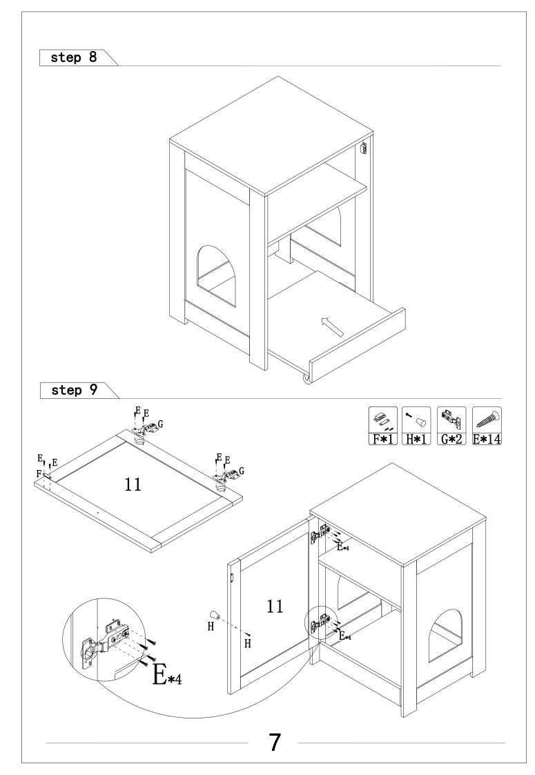
**EN\_**It may be necessary to adjust the hinges so that the doors align. Use the instructions below as a guide.
