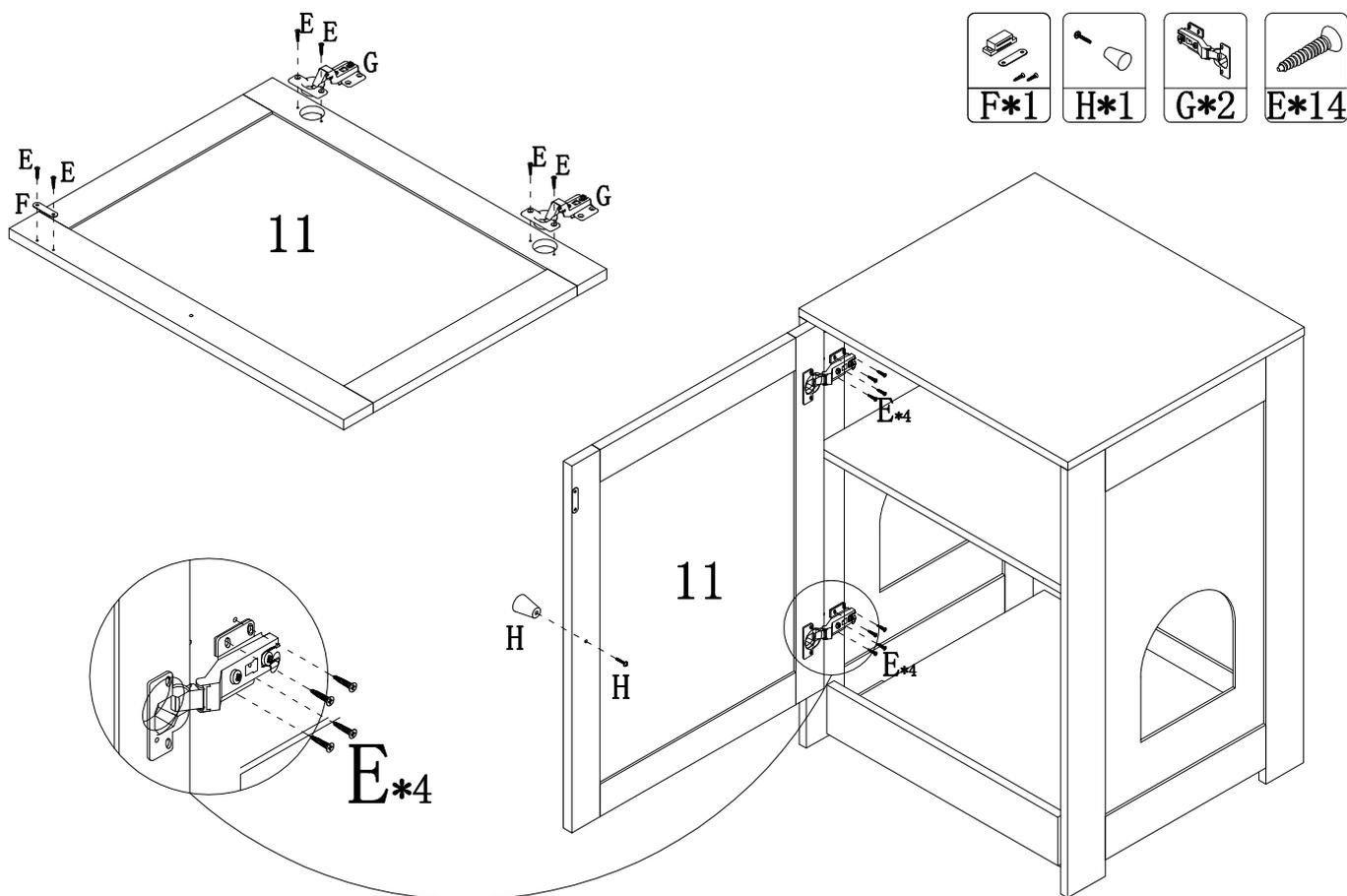
**EN** It may be necessary to adjust the hinges so that the doors align. Use the instructions below as a guide.
