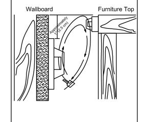
Important: Make sure the brackets are firmly attached to the wall stud and furniture frame and the safety strap is snug.
