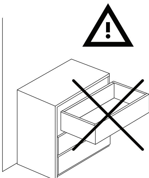
Do not defeat or remove the drawer interlock system. It is important stability and safety system.
