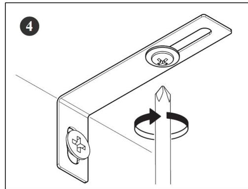
Screw the safety bracket to the wall stud:
