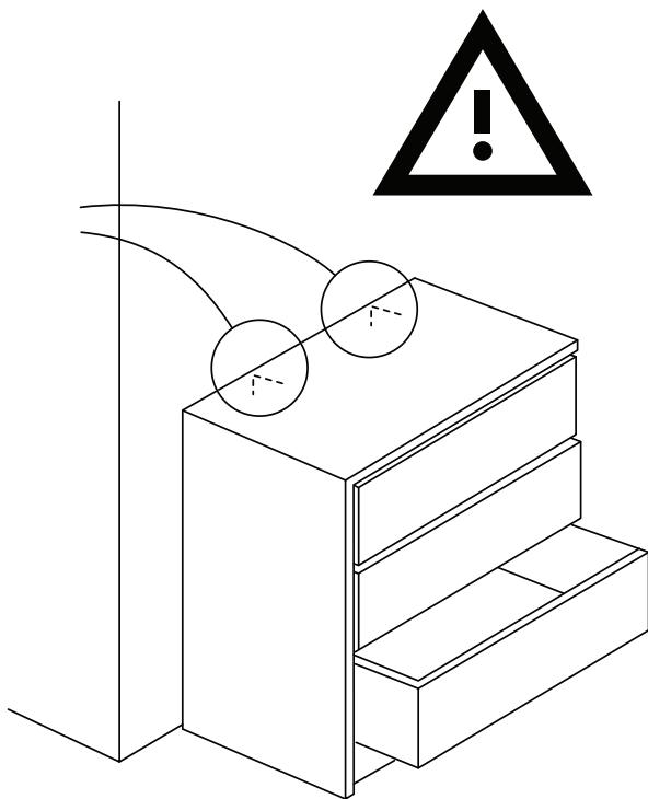
Never use the unit without the interlock system installed following the instructions
