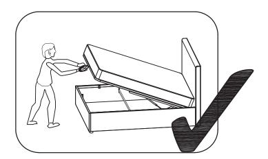
Attention: Do not tighten the screws before completing the entire installation. If you have any difficulty with the installation process, please feel free to contact us.
