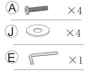
Fix the Headboard legs(20L) / (20R) To the headboard(1) With Bolts (A) and Flat Washer (J) by using Allen key (E), you can chose the holes a and b or b and c .
