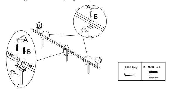
Fix the Center support bar 10 to the Center support bar fittings G with Bolts B by using Allen key A
