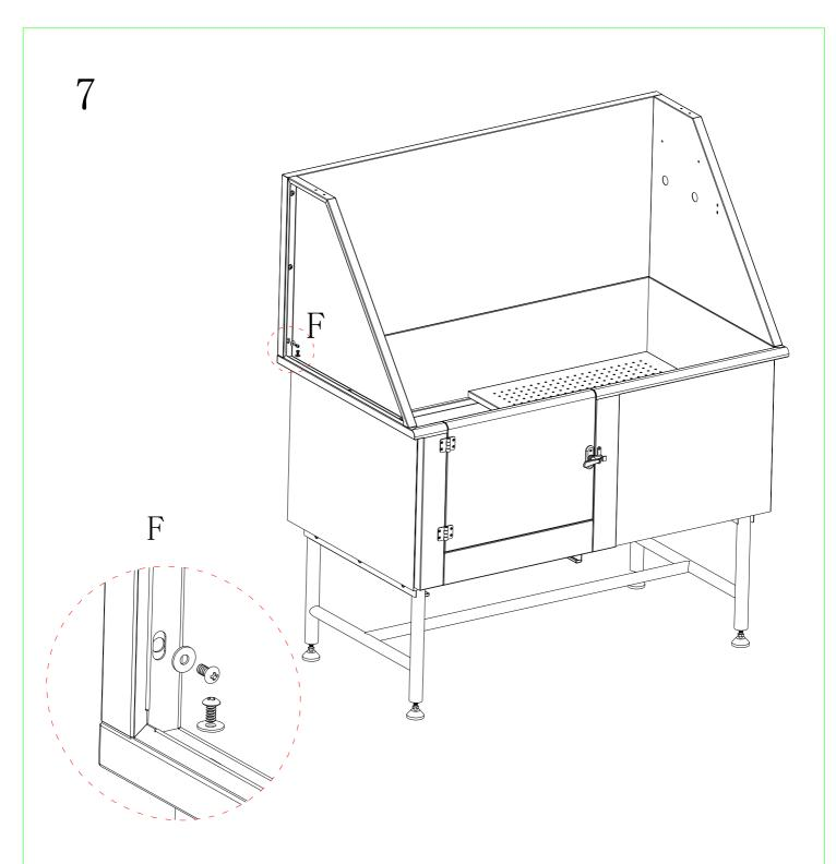
Step 7: Install the left and right baffles with M5 screws and spacers, the bottom edge is fixed to the box and the back edge is fixed to the baffle, all the screws are fixed slightly first to make sure the positions are all aligned before tightening.
