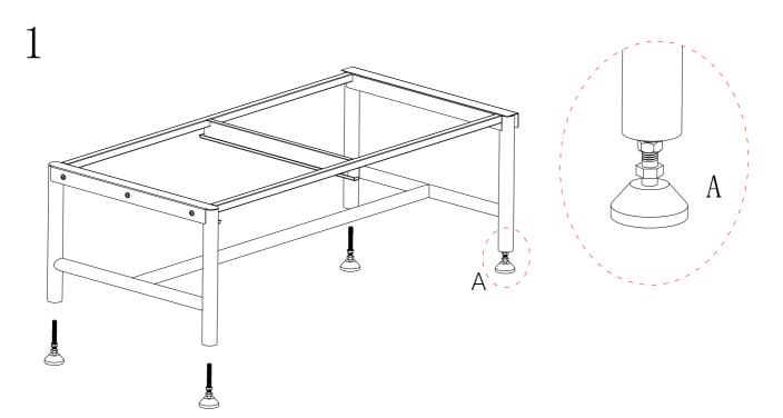
Step 1: Screw the adjusting feet into the frame legs and adjust the 4 feet for balance, then turn the nuts until they are torqued.
