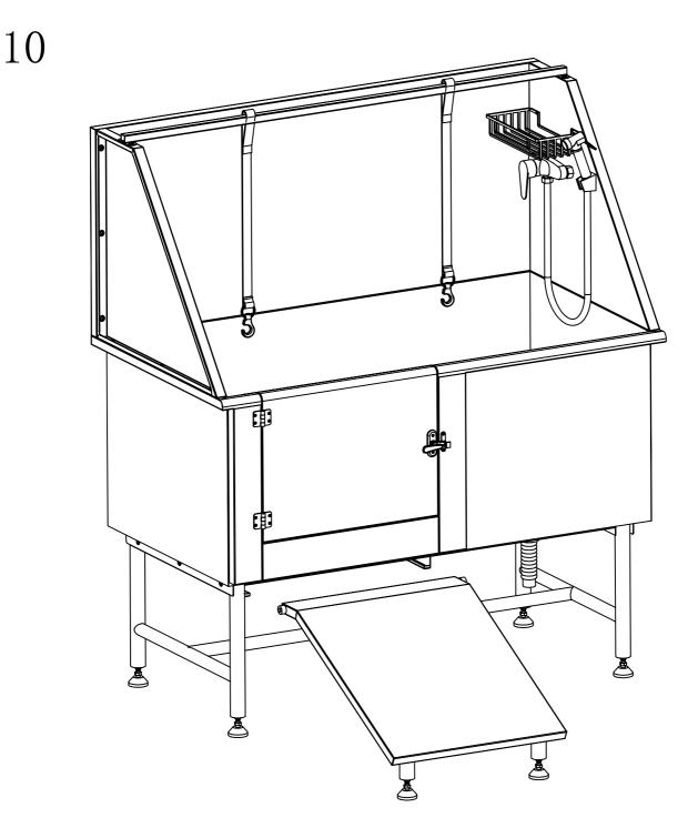
Step 13: To install the pedal, first screw the two feet of the pedal on the adjusting feet and adjust the balance, then push the pulleys on the left and right side of the pedal into the slide rail track on the bottom frame, push the pedal into the bottom frame, and you can pull out the pedal when you use it.
