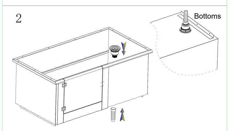
Step 2: Install the drain and drain hose into the box and tighten.
