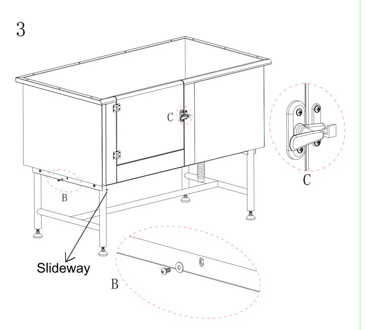
Note: The bottom frame has a slide groove on one side, which is used to install a foot pedal to facilitate pets to go up and down, when the box and the frame are installed, the slide groove should be on the same side as the door, please pay attention to the direction of the installation to avoid installation errors.
