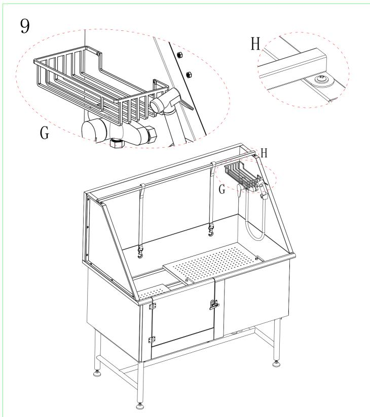
Step 11: Install the soap holder, use M4 screws with nuts to fix the soap holder on the side panel.
