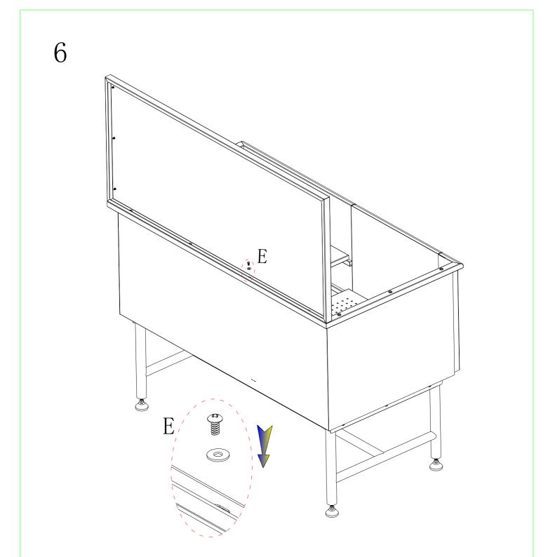
Step 6: When installing the rear bezel, note that the back of the bezel is slightly secured with M5 screws and spacers, but do not tighten.
