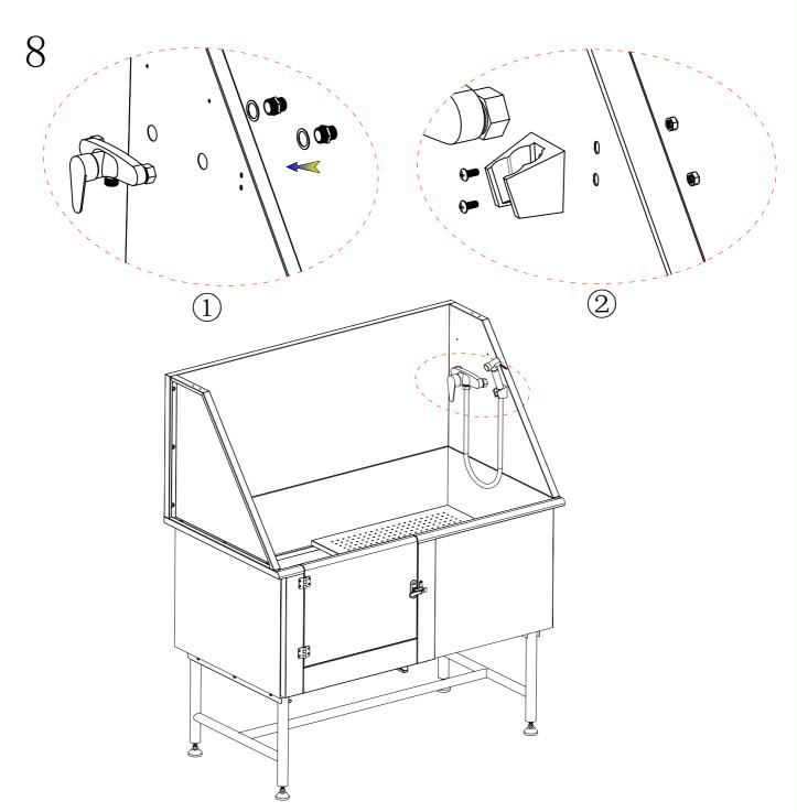
Step 8: Install the on/off valve by running a brass fitting through the right side panel hole, along with a 35mm stainless steel gasket, and tightening the on/off valve nut on the other side.
