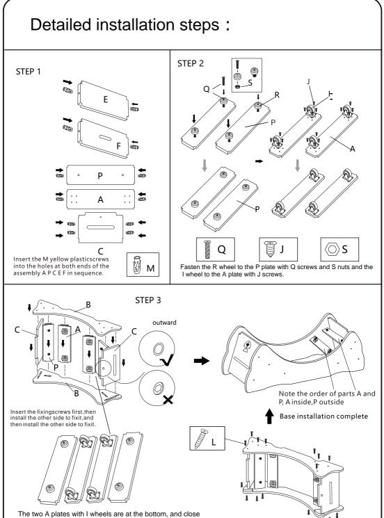
to the A plates are the two P plates with R small wheels.
