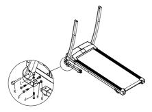
**Step 4:** First insert the Electric watch rack into the column in the direction of the arrow, and then fix the Electric watch rack on the column with E # M8 flat washers (4 pieces) and D # M8 \* 16 (4 pieces) (as shown in the figure). Note: B # 6mm Hex key is required here.
