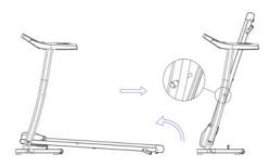
Product deployment: Use your hand to pull out the K # pin on the column, then lower the running table to make it come into contact with the ground to deploy the product. Then, insert the K # pin from the bottom of the column into the hole in the iron plate at the front end of the running table.
