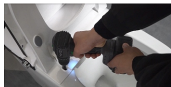
7. Unscrew the screws on the toilet seat
