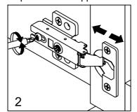
3.Use the screw at the front end of the hinge to adjust the left and right position of the door panel(ensure that the left and right sides of the door panel are in the same plane as the upper and lower panels).4.After completing these three steps secure the other two screws on the hinge.
