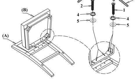
DO NOT TIGHTEN BOLTS UNTIL COMPLETELY ASSEMBLED.
