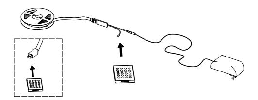
3. Align romote controller to the RGB Control box to adjust the color mode
