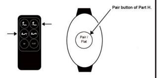
Simultaneously press and hold the HEAD DOWN, FOOT UP, PAIR buttons on the remote and Part H cable until the buzzer of control box sounds three times.
