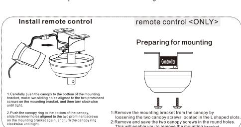
This will enable you to remove the mounting bracket
