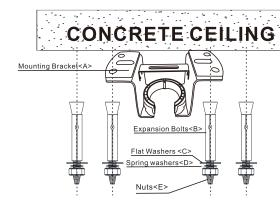
Note: According to the ceiling of different materials, use different screws to fix the hanging bracket. Don't fix the hanging bracket on the wood ceiling less than 12MM to prevent danger caused b loosening of screws.
