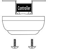
I:Remove the mounting bracket from the canopy by loosening the two canopy screws located in the L shaped slots
