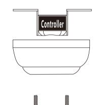
Remove the mounting bracket from the canopy by loosening the two canopy screws located in the L shaped slots. Remove and save the two canopy screws in the round holes. This will enable you to remove the mountingbracket
