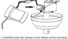
bracket, make two sliding holes aligned to the two prominent screws on the mounting bracket, and then turn clockwise 2. Push the canopy ring to the bottom oft he canopy, slide the inner holes aligned to the two prominent screws on the mounting bracket again, and turn the canopy ring clockwise until tight.
