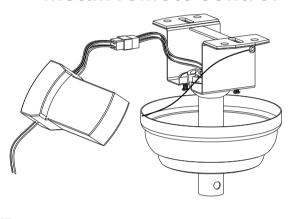
Carefully push the canopy to the bottom of the mounting bracket, make two sliding holes aligned to the two prominent screws on the mounting bracket, and then turn clockwise
