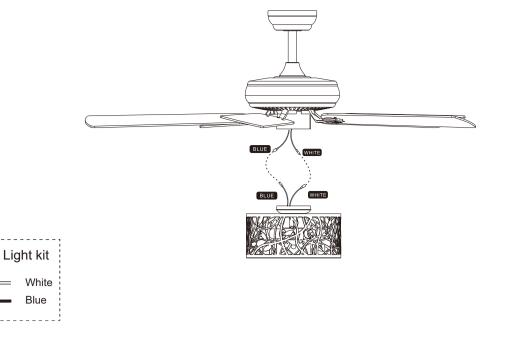
☐ Insert the "white" line in the switching box of the motor into the "white" line of the light and tie insulated rubber tape.
