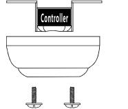
I:Remove the mounting bracket from the canopy by loosening the two canopy screws located in the L shaped slots 2:Remove and save the two canopy screws in the round holes.
