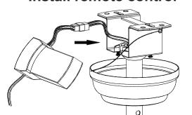
1. Carefully push the canopy to the bottom of the mounting
