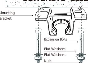
For concrete ceiling, use the percussion bit with diameter 8mm to drill holes according to the length of expansion screws. Then use the attached expansion screws to fix the hanging bracket onto the ceiling (selection is made according to actual requirements of the customers).
