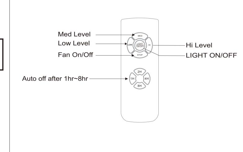
LOW FanSpeed Low Level MED FanSpeed Middle Level
