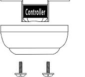
I:Remove the mounting bracket from the canopy by loosening the two canopy screws located in the L shaped slots
