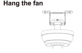
☐ Lift the fan motor assembly up to the mounting bracket and seat the hanger ball in the mounting bracket socket.Rotate the fan motor assembly until the check groove drops into the registration slot and seats firmly. The downrod should not rotate if the is done correctly
