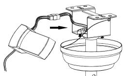
1. Carefully push the canopy to the bottom of the mounting bracket, make two sliding holes aligned to the two prominent screws on the mounting bracket, and then turn clockwise 2. Push the canopy ring to the bottom oft he canopy, slide the inner holes aligned to the two prominent screws
