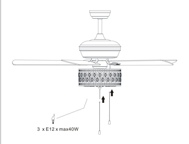
1.knot the chain to the excessive switch chain (pull rope only) 2.knot the appointed crystal to the appointed place. 3.intall the bulb to the lamp holder.
